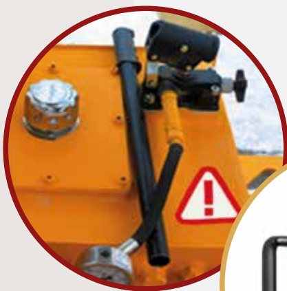
Emergency Hand Pump
